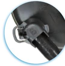
When required, locking distributor terminals rotate to proper clock position. This eliminates crossed wire issues and provides a clean installation.
