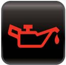
**Oil Pressure Warning:** If this light stays lit it indicates loss of oil pressure. Immediately check oil level and pressure.
