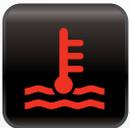
**Coolant Temp Warning:** Indicates temperature has exceeded normal limits. Check coolant level, fan operation, radiator cap, coolant leaks.
