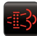
**DPF Light (Diesel):** The diesel exhaust particulate filter has failed its test and needs to be serviced.
