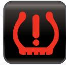
**TPMS (Tire Pressure Monitoring System):** Indicates the tire pressure monitoring system has found a tire with low air pressure or there may be a sensor malfunction. Check tire pressure. Some vehicles will allow manual reset of TPMS warning light and others will require professional diagnosis. Refer to owner's manual.
