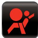
**Airbag Fault:** If this light stays illuminated after starting it indicates that the vehicle has found a fault in the airbag system and the computer has set a code. Professional repair of the supplemental restraint system is highly recommended.
