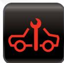
**Service Vehicle Soon:** Typically indicates a lighting or other electrical problem that is controlled by the BCM (body control module). Check all lights, head lights, turn signals, brake lights, and hazard lights. This symbol may also be used to warn driver of a traction control problem, or a communication problem between modules.
