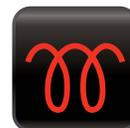
**Glow Plug (Diesel):** On diesel vehicles this light indicates that the engine's glow plugs are warming up and the engine should not be started until this light goes out.
