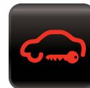
**Security Alert:** If the symbol lights momentarily it may mean that the ignition switch is locked and will need the proper transponder-equipped key to re-start. If the symbol is visible when the vehicle is on, then it typically indicates a malfunction in the security system.
