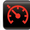
**Cruise Control:** Indicates that cruise control is set during driving.
