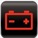
**Battery/Charging Alert:** Indicates voltage level is below normal level and the vehicle's charging system is not functioning properly. Check battery terminals, alternator belt, and battery condition.
