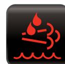
**DEF Light (Diesel):** The diesel exhaust fluid reservoir is low on fluid.
