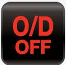
**Overdrive Light:** This symbol indicates that the vehicle's overdrive system has been manually turned off. Typically the overdrive system is controlled by an on/off switch.
