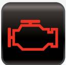
**Check Engine or Malfunction Indicator Light (MIL):** Indicates the engine computer has set a Diagnostic Trouble Code (DTC). Usually requires diagnosis with a professional scan tool.
