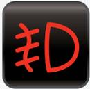
**Fog Lamp:** Indicates that the vehicle's front fog lamps are illuminated.
