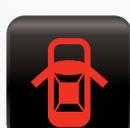
**Door Ajar:** Indicates that a door (including hood and trunk) is not closed. Open and close all doors, including hood and trunk. If vehicle is left in this condition overnight it can drain the battery.
