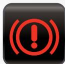
**Brake System:** Indicates one of three possible conditions: parking brake is on; problem with the braking system/brake fluid is low, or ABS problem. Check brake fluid and make sure the parking brake is fully released. If the problem is in the ABS system, it may need a professional diagnosis.
